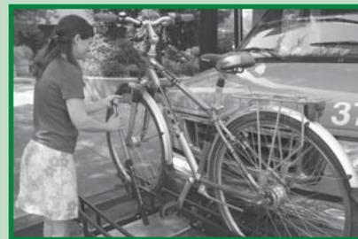
*Pull the support arm out and up over the front tire to secure the bike. Use your bike lock to secure the bike to the rack.*
