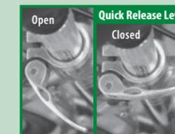
**WHEELS:** Wheel nuts and quick release levers need to be tight, and the wheel should not wobble. Check for loose or broken spokes. Lift each end of your bike, spin the wheel to ensure your brakes do not rub the tire or dive into spokes.
