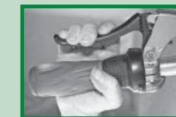
**BRAKES:** While standing next to your bike, push your bike forward while squeezing each brake lever individually to be sure they are capable of locking up the wheel. Inspect pads for wear; replace
